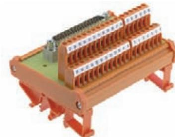
Users have a choice between screw, tension clamp or spade connections for connecting actuators and/or sensors. As an option, interface units can also integrate additional functions such as status indicator, signal disconnector, fuses or shielding. Identification systems make it easier to trace the signals to the corresponding element.
