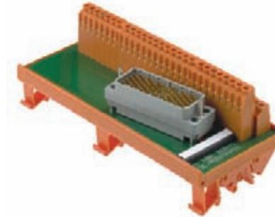
Weidmüller's passive interface units are used for adapting hermaphrodite ELCO multi-pole connectors, for input and output, to screw terminal systems. The hermaphrodite contact is a fork-type contact that is identical in design on both sides of the connection, but with one fork turned through 90° to engage with the other.
